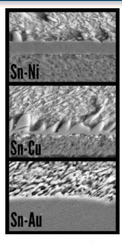
solder joint you cannot see from the outside. This is the weakest non compliant region of a solder joint the IMC (Intermetallic Compound zone)
