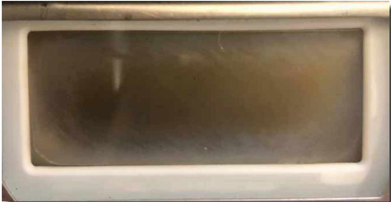
Figure 1. LCD with vinegar syndrome
