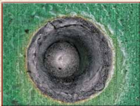
Figure 1: Appears to be a cracked solder joint
