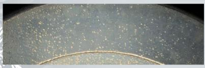
Figure 2. Tin plating treated to prevent sulfation
